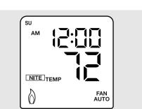
Figure 3: Default Display after Reset and Initial Power-Up
